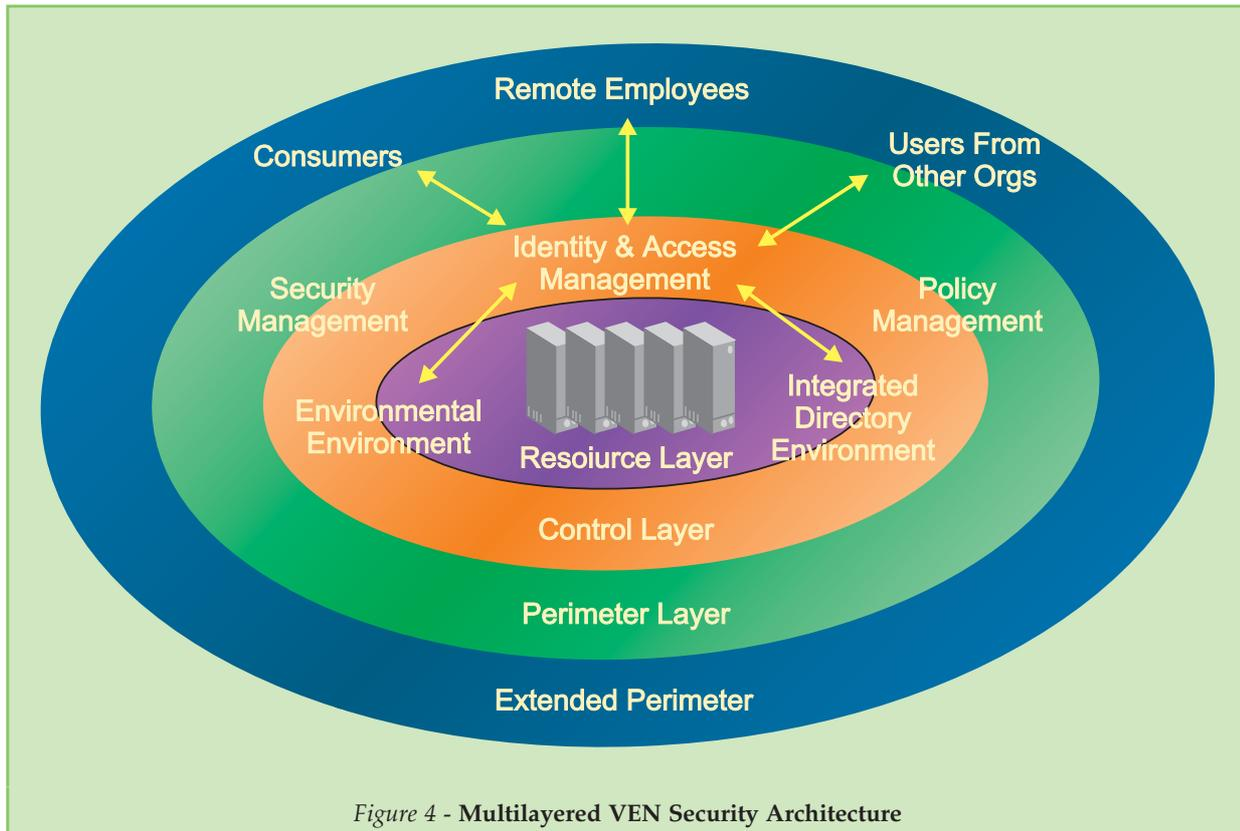
Figure 4 - Multilayered VEN Security Architecture
